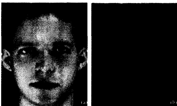
图 2 人脸图像(a)和其强度响应的结果(b) Fig.2 Human face image (a) and its magnitude response (b) by a Gabor filter
